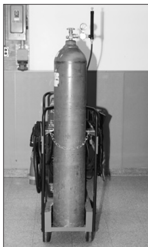
Figure 3.28 Cylinder is securely chained in a safe operating condition with a running gear to allow ease of moving the power source and related equipment.
