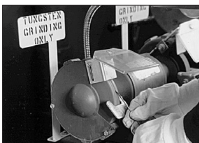
Figure 4.10 Tungsten electrode preparation.
