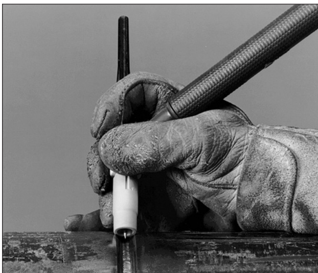
Figures 8.11 and 8.12 Demonstrations of two common methods of grasping the torch for pipe welding. There is no single “correct” method of doing this and each welder is encouraged to experiment with several different methods until one is found that is most comfortable, and results in satisfactory welds.
