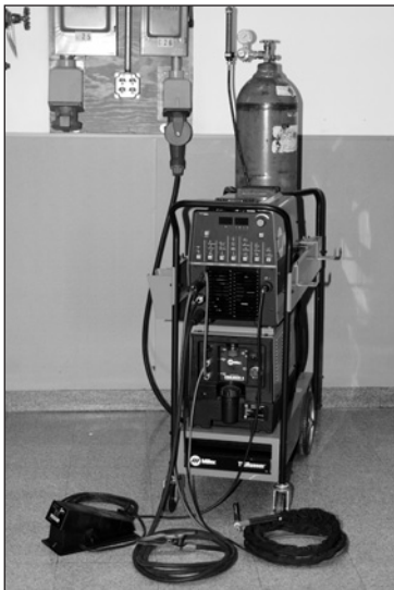
Figure 3.1 GTAW power source plugged into wall connection. Primary connection to the commercial power.
