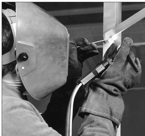
Figure 8.10 Welding in the overhead position.
