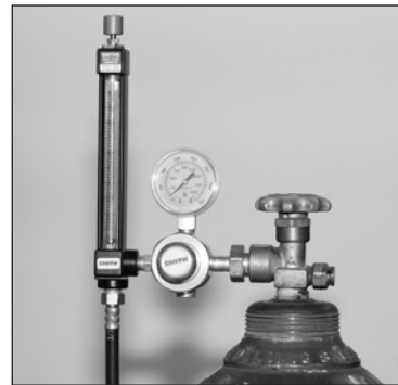
Figure 4.15 The regulator/flowmeter regulates the flow of shielding gas from the cylinder to the welding torch. This meter displays the amount of pressure in the cylinder as well as the rate of flow.
