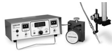
Figure 3.38 A seam tracker for maintaining the arc and joint alignment.
