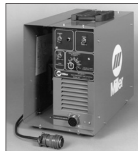
Figure 3.21 A high-frequency arc starter and stabilizer.
