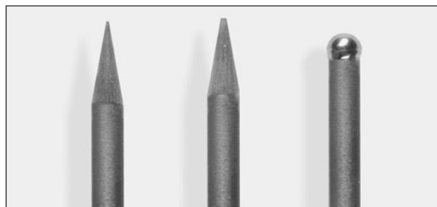
Figure 4.6 The ball diameter should never exceed 1.5 times the electrode diameter. Pointed tungstens are as noted.
