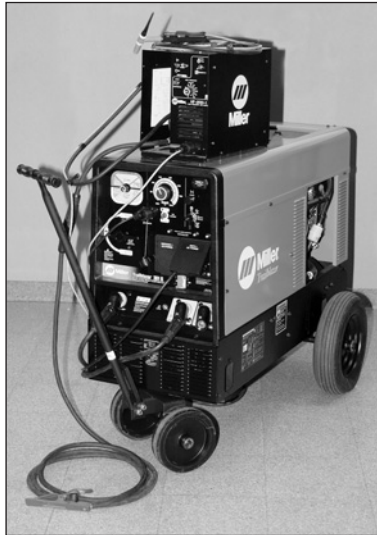
Figure 3.6 A multiprocess engine-driven welding generator capable of AC and DC GTAW welding when fitted with an optional high-frequency arc starter.
